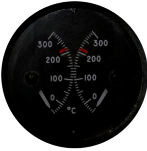
WING ANTI-ICING HEATER AIR TEMPERATURE INDICATOR
