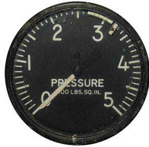
HYDRAULIC PRESSURE GAUGE Red radial at 3200 PSI Green arc from 2600 PSI to 3100 PSI
