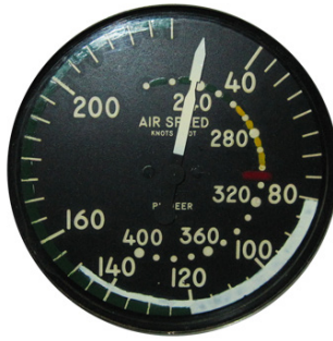
AIRSPEED INDICATOR (for 93,200 pound airplane)
