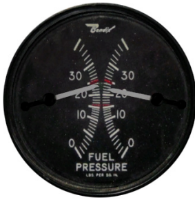
FUEL PRESSURE INDICATOR Red radial at 16 PSI Green Arc from 22 PSI to 24 PSI Red Radial at 25.5 PSI
