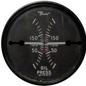
OIL PRESSURE INDICATOR Red radial at 50 PSI Green arc from 75 PSI to 95 PSI Red radial at 110 PSI
