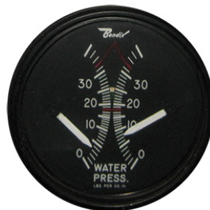
W / A PRESSURE GAUGE Red arc from 21 to 32 Green arc from 21 to 23
