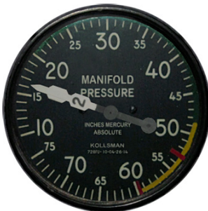
MANIFOLD PRESSURE GAUGE Red radial to 55 in. Hg. Green arc from 20 in. Hg. to 46 in. Hg. Yellow arc from 46 in. Hg. to 55 in. Hg. Long red radial at 59.5 in. Hg.
